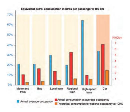
As regards the greenhouse effect and global warming, vehicles with lower capacity and driven by combustion engines produce the highest quantities of CO2 per passenger. Passenger cars are particularly to blame for this due to their high mass-performance ratio.
