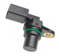
Crankshaft position and speed sensor: A Hall type sensor reads the speed and angular position of the engine's crankshaft in order to be able to initiate the cylinder deactivation system and manage both the ignition and injection times.
