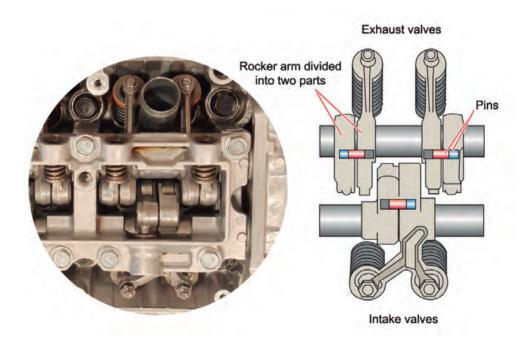
The system is based on the use of composite rocker arms (divided into two parts) which are connected or disconnected by means of hydraulically controlled pins. One part of the rocker arms works on the valves, while the other receives the camshaft movement through a roller. At rest, the pins located inside the rocker arms keep both parts connected, in such a way that the rocker arms tilt on their axes to transmit the profile variation of the cams to the valves.
