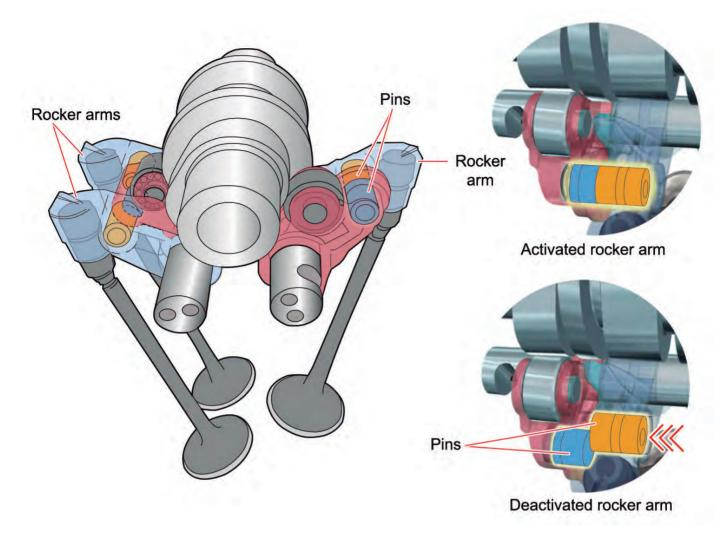
In addition, a sequential fuel injection system is used in this engine that cuts the fuel supply to the cylinders that are mechanically "deactivated". This solution corrects another of the defects of the system used by Cadillac, which was the condensation and accumulation of fuel in the inlet lines of the deactivated cylinders that occurred in the carburettor fed V8-6-4 engine.
