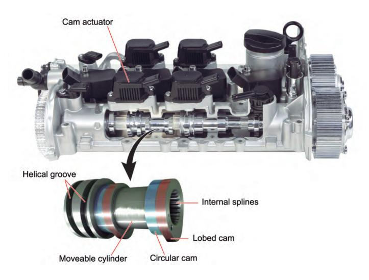
The cam cylinder is fixed in a specific position by means of a spring and ball retainer and its axial displacement is achieved by the ac-
