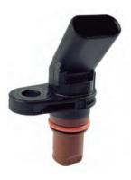
Intake manifold pressure and temperature sensor: The pressure in the intake manifold is very variable during the regulation of the cylinder activation and deactivation. This sensor allows the position of the throttle to be regulated and to calculate the effective filling of the cylinders.
