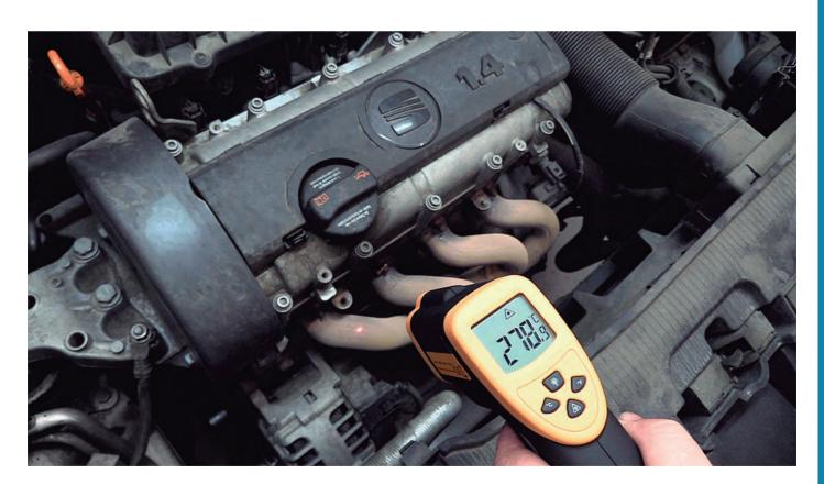
The oxidation reaction of the CO and HCs is endothermic, so the gases are heated as they pass through the catalytic converter. The outlet-inlet temperature difference of the catalytic converter must be between 50-70°C, provided that the mixture ratio is acceptable, the quantity of CO at the catalytic converter inlet is greater than 0.4% and the  $\rm CO_2$  greater than 13%.
